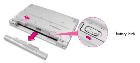
4. To install the battery again, insert the battery into the battery compartment of the system and slide the right battery latch in the direction of **closed**( $\triangle$ ) to fix the battery.
